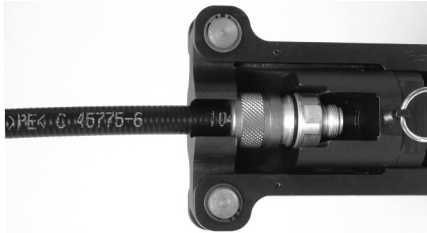
Figure 5 – Connector Properly Nested In the Frame's Counterbore
